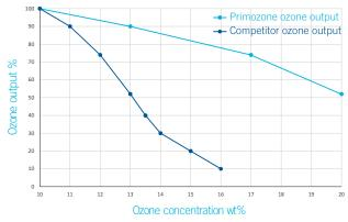
The graph shows that Primozone's ozone technology has more than 7 times the production capacity at higher ozone concentrations than competitive technology.
